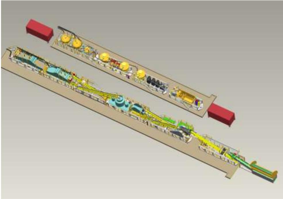
Figure 7: Python 500 installed on surface in a “U” shape.
