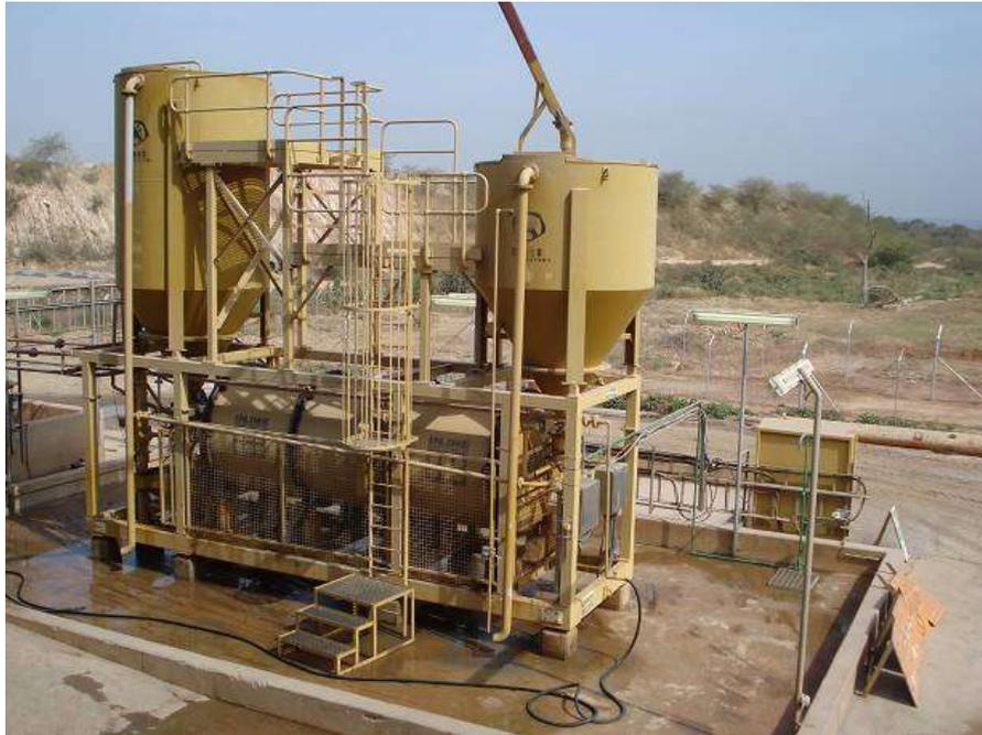
Figure 10: Batch ILR within bunded area.
