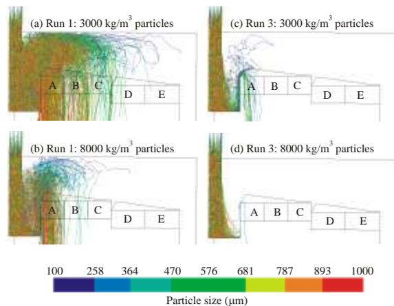
Figure 2: CFD modelling output example – particle tracking
