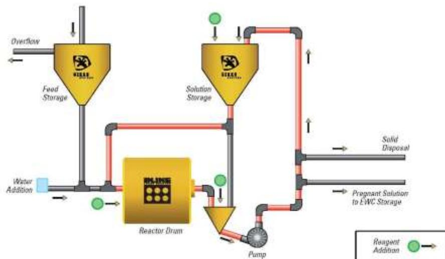
Figure 9: Batch Reactor Flow Diagram
