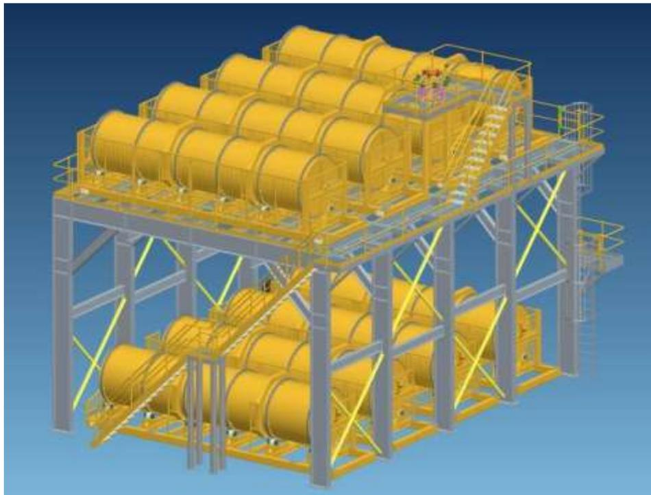
Figure 12: Continuous ILR Leaching System
