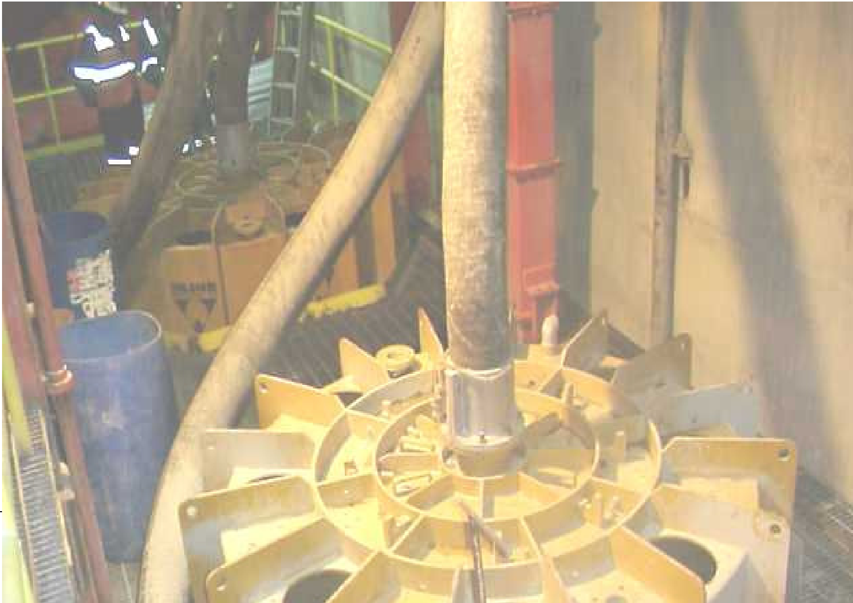
Page 12 Figure 7: View of Gekko IPJ2400 Lid Platform Showing the Feed Pipes from the Rotating Distributor.
